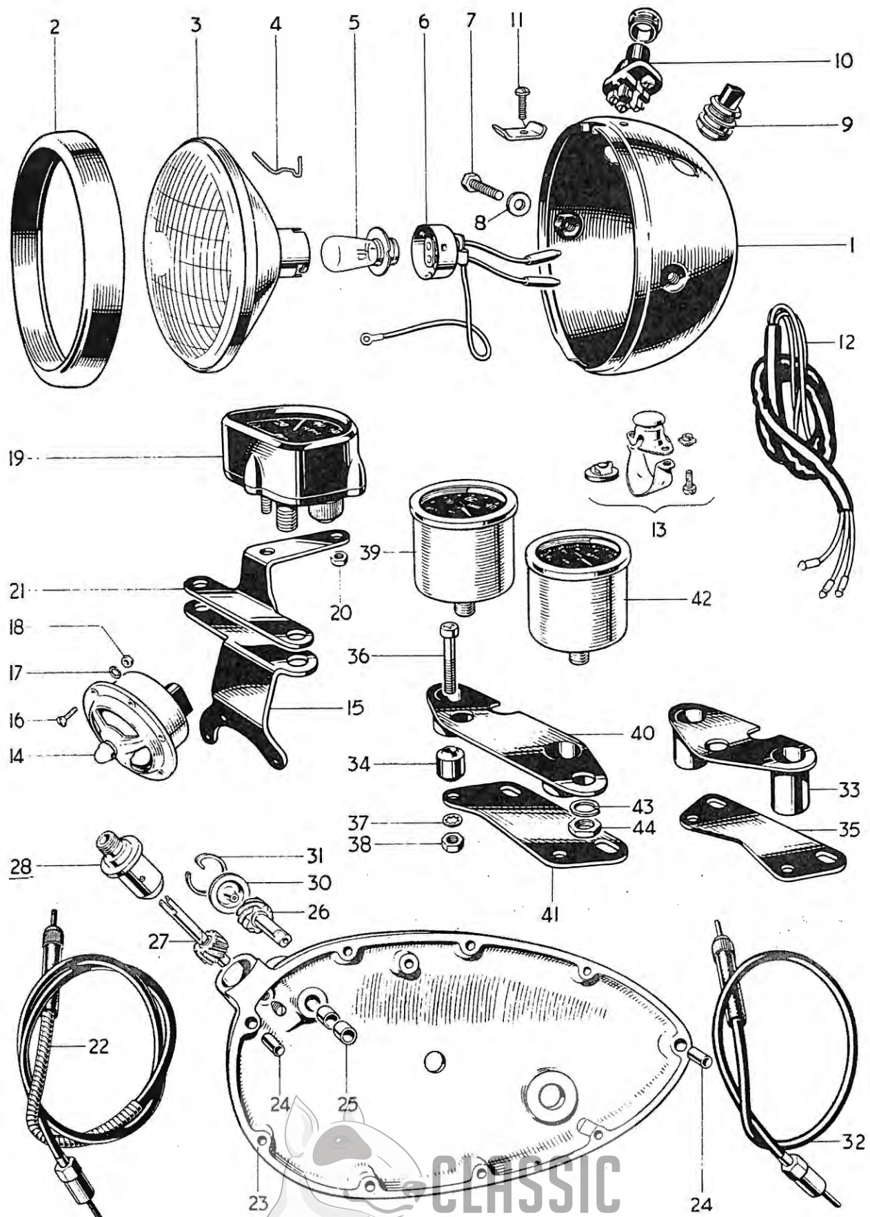
Fig. 13. T20SL HEADLAMP, TACHOMETER, Etc.
